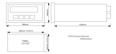
The Indicator must be installed in a dry, non-hazardous location. A panel cut out of 92 mm (+1.0/0.0 mm) x 45 mm (+1.0/0.0 mm) is required. The depth of the Indicator is 125 mm but extra provision must be allowed for cable connections. A single fixing clip, behind the unit, retains the Indicator. To install, simply insert the Indicator into the cut out and fit the clip to hold the Indicator in place.
