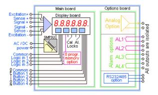
The Indicator can accept full scale input voltages of either up to +/- 40 mV (foil strain gauges) or up to +/- 400 mV (semi-conductor strain gauges) for full display with selectable decimal point position and scaling, and a zero offset for both positive and negative sensing.
