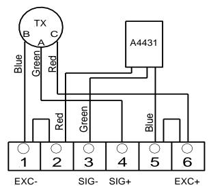
Connections for two Cleveland Kidder Classic Semi-Conductor Transducer (two Half Bridge Transducer)
