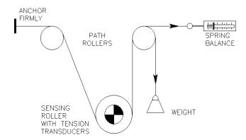
To calibrate the LETIX indicator correctly a spring balance (or weights) to provide the required tension force and some flat strapping or similar to simulate the web will be needed.
