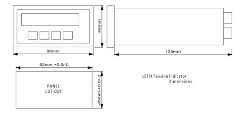
The Indicator must be installed in a dry, non-hazardous location. A panel cut out of 92 mm ( $\pm 1.0/0.0 \text{ mm}$ ) x 45 mm ( $\pm 1.0/0.0 \text{ mm}$ ) is required. The depth of the Indicator is 125 mm but extra provision must be allowed for cable connections. A single fixing clip, behind the unit, retains the Indicator. To install, simply insert the Indicator into the cut out and fit the clip to hold the Indicator in place.
