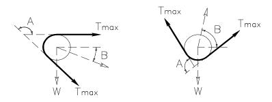
The formula for calculation of the transducer maximum working force (**MWF**) or force rating allows a 100% overload for tension transients or a tight edge to the web.
